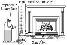
Figure 35 - Checking Gas Joints for Propane/LP Gas Fireplace
